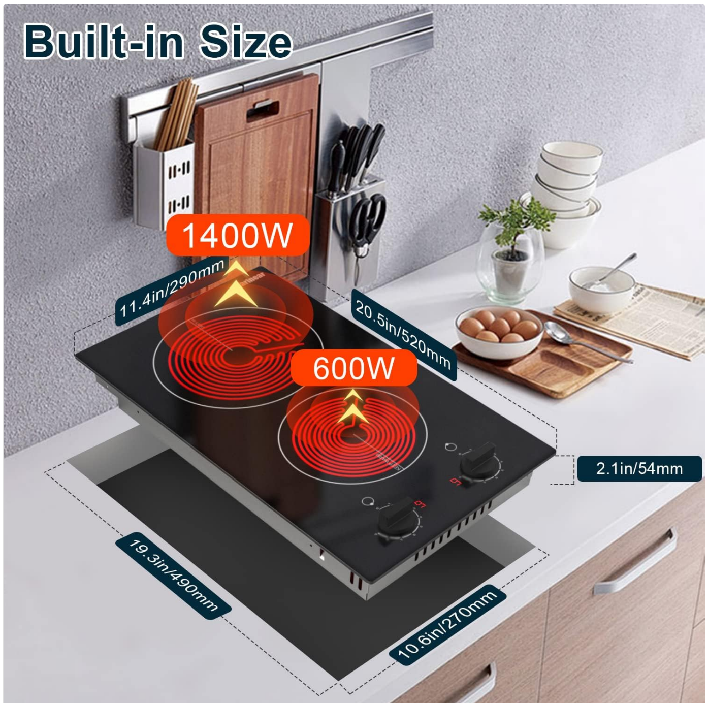
Figure 3.2: Built-in Size Diagram. This diagram provides the precise measurements for installing the cooktop into a counter, including the overall dimensions of 20.5 inches (520mm) by 11.4 inches (290mm) and the cut-out size of 19.3 inches (490mm) by 10.6 inches (270mm). It also indicates the power of each burner: 1400W and 600W.
