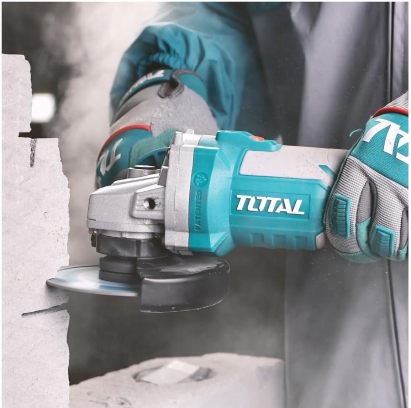
Figure 4.3: Angle grinder in use for cutting stone.
