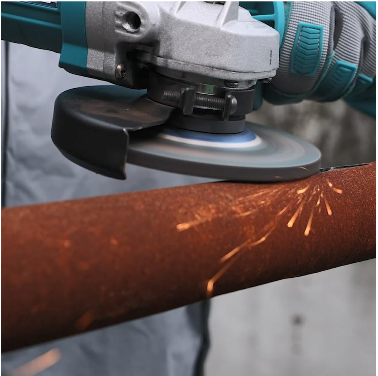
Figure 4.4: Angle grinder in use for grinding metal.
