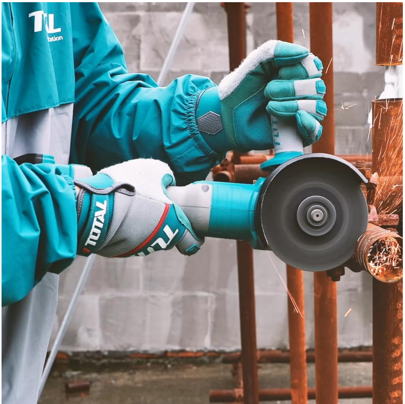
Figure 4.2: Angle grinder in use for cutting metal.
