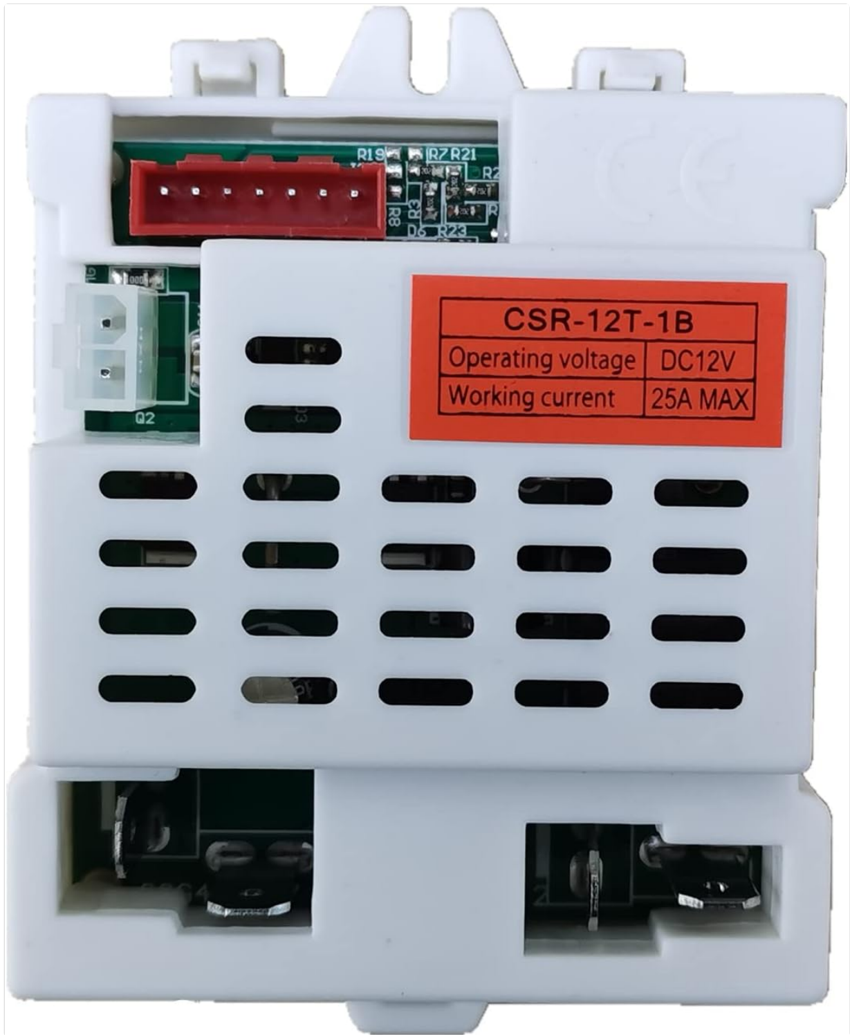
Figure 1: Top view of the CSR-12T-1B 12V Control Box. This image displays the main control unit with its identification label, operating voltage (DC12V), and maximum working current (25A MAX).
