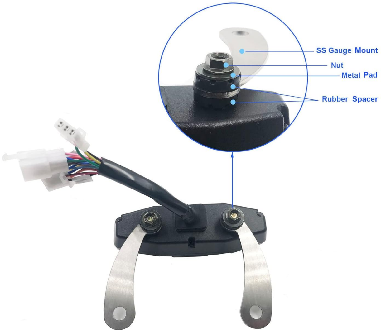
Figure 5.2: Mount Installation Diagram.
