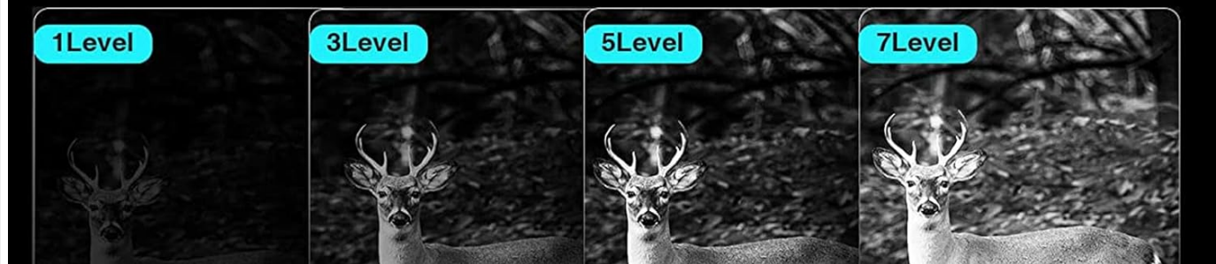
Image: Depicts a deer in a dark forest, viewed through the monocular, with examples of different IR levels (1, 3, 5, 7) showing increasing clarity.
