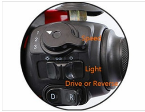
Image: Close-up of the right handlebar showing controls for speed selection (1, 2, 3), light switch, and drive (D) or reverse (R) selector.
