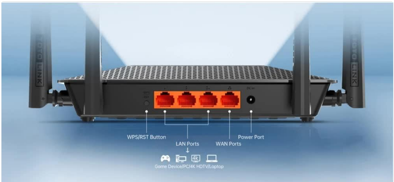
Figure 3.4: TOTOLINK A3300R Router Port Diagram. This diagram clearly labels the WPS/RST button, LAN ports, WAN port, and Power port on the rear of the router.
