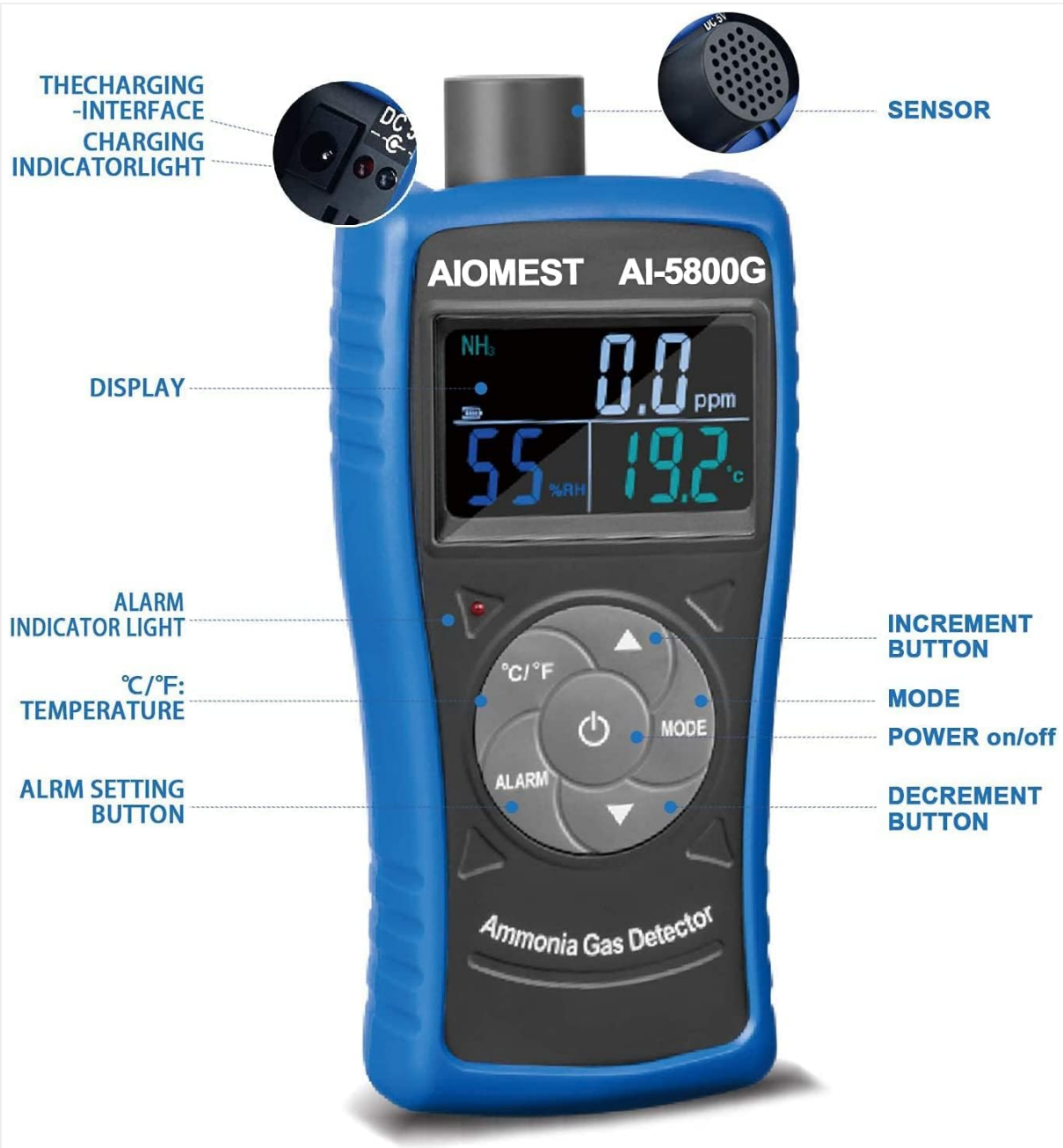
Figure 2.1: Front view of the AIOMEST AI-5800G Ammonia Gas Detector with key components labeled.
