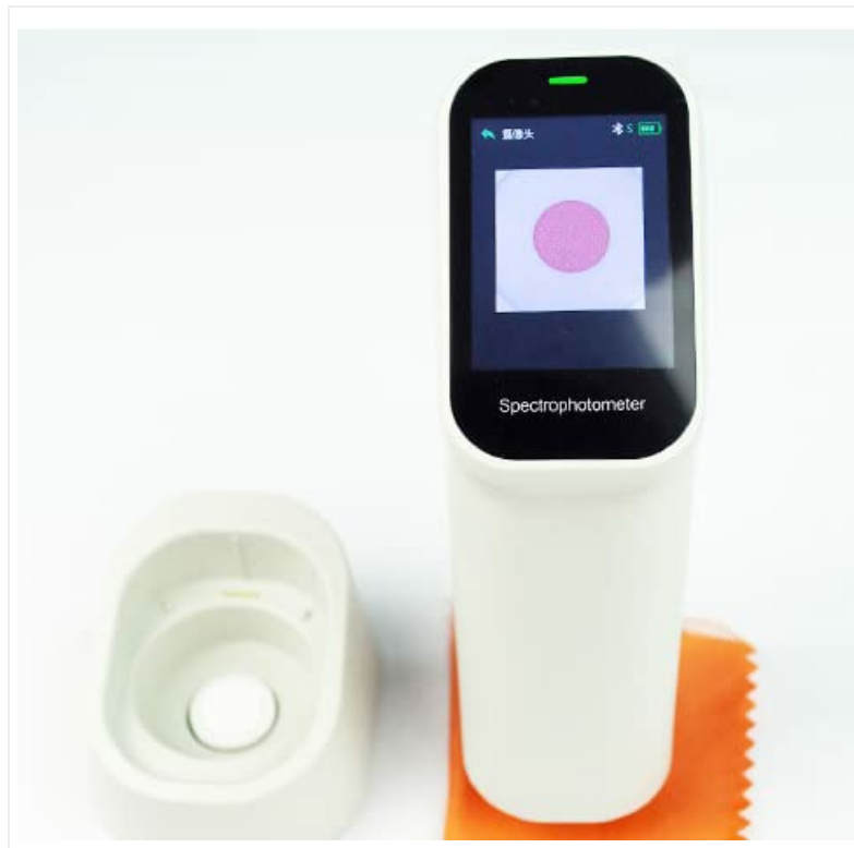
Figure 3.2: The colorimeter placed in its charging base, with the screen displaying measurement data.
