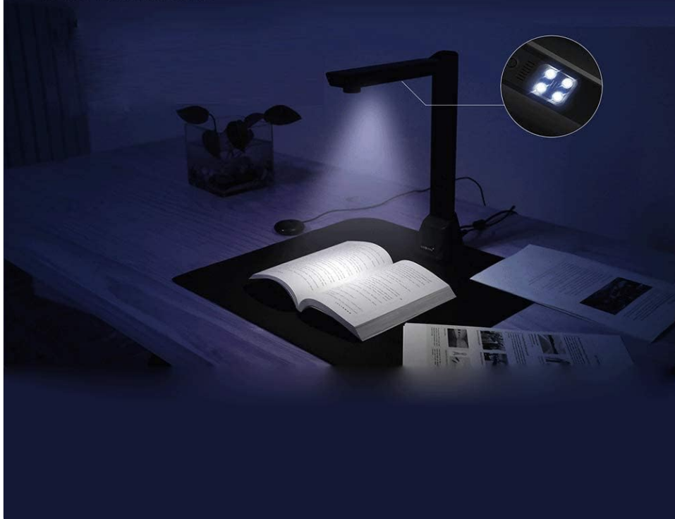
Figure 4.6: The VK16 features intuitive lighting controls with a built-in adjustable LED lamp to ensure high-quality scans in any lighting condition.
