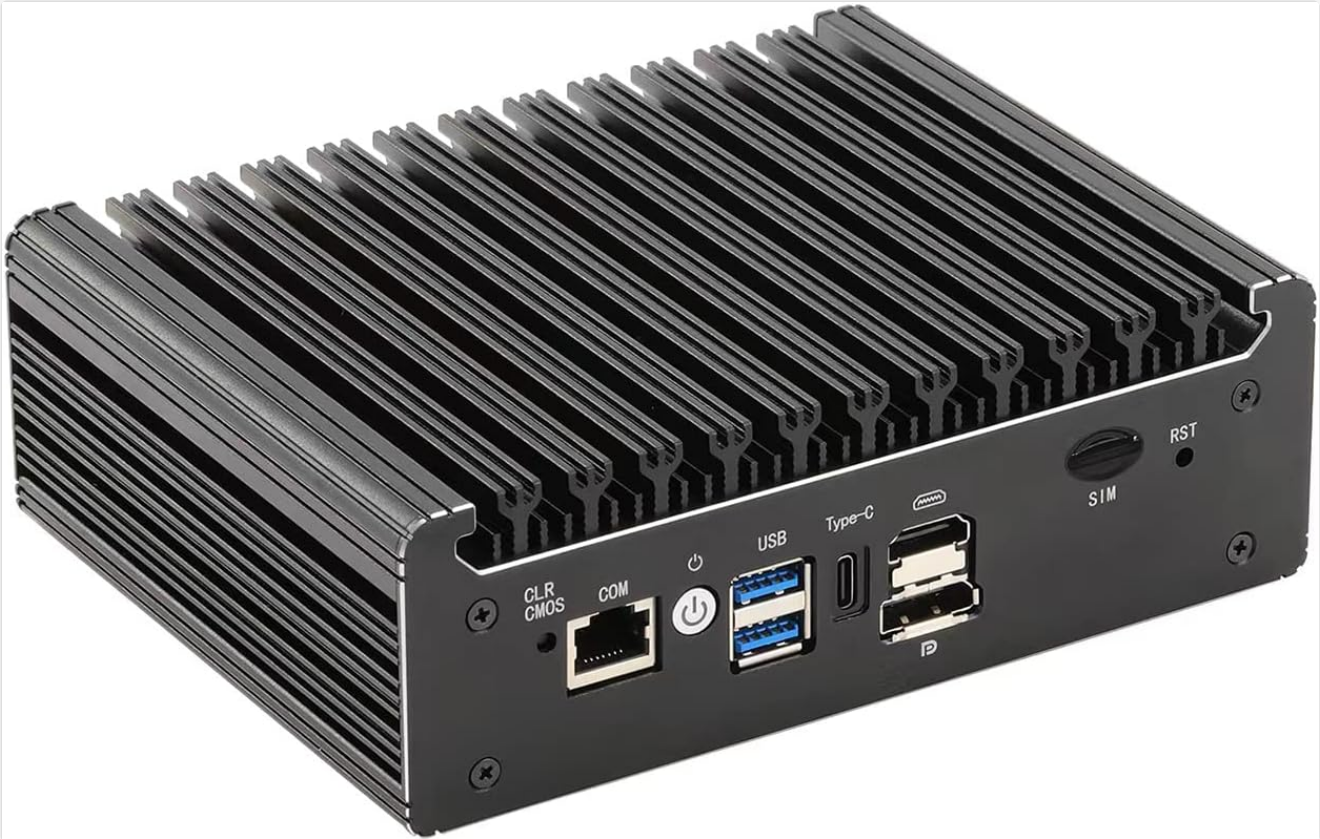
Figure 2: Front Panel I/O
