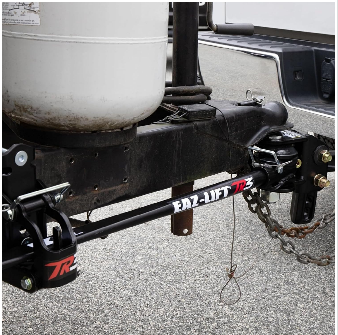
Image: The Eaz-Lift TR3 hitch installed on a trailer, demonstrating the connection points and overall setup.
