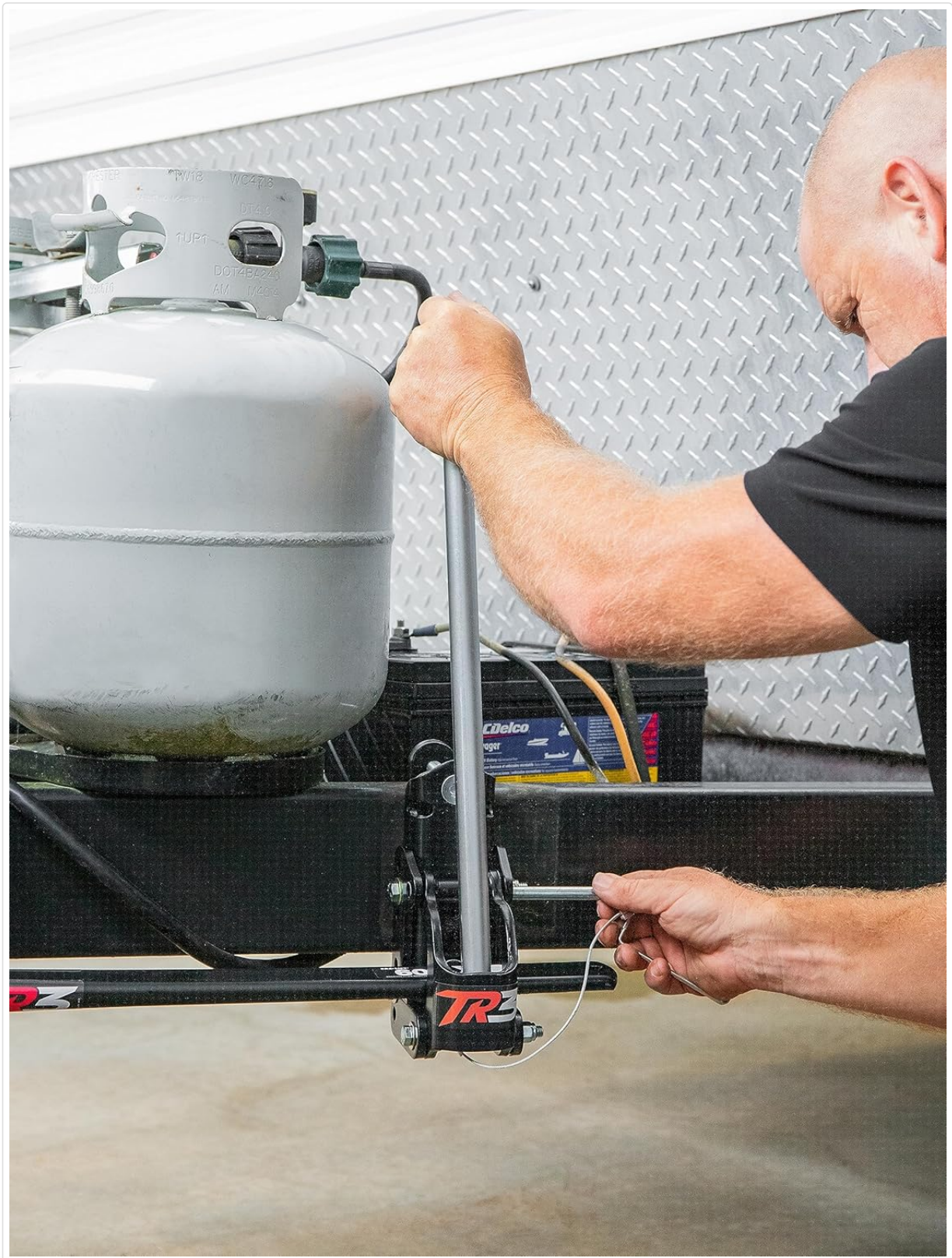
Figure 3.4: An individual using a leverage bar to secure a spring bar into its hookup bracket, illustrating the force required for proper engagement.
