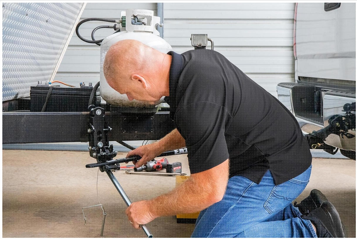
Figure 3.3: An individual kneeling to make adjustments to the spring bar connection at the trailer frame, demonstrating the setup process.
