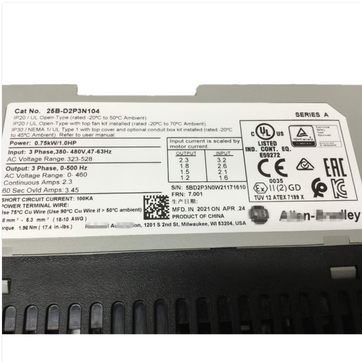
Figure 3.2: Product label on the Allen-Bradley PowerFlex 525 AC Drive. This label provides critical information such as the catalog number (Cat No. 25B-D2P3N104), series (Series A), power rating (0.75KW/1.0HP), input voltage (3-Phase, 380-480V, 47-63Hz), output voltage (3-Phase, 0-500 Hz), and various current ratings. It also lists certifications (UL, CE, EAC, RCM) and manufacturing details, including the date of manufacture (MFD. IN 2021 ON APR. 24) and country of origin (PRODUCT OF CHINA).
