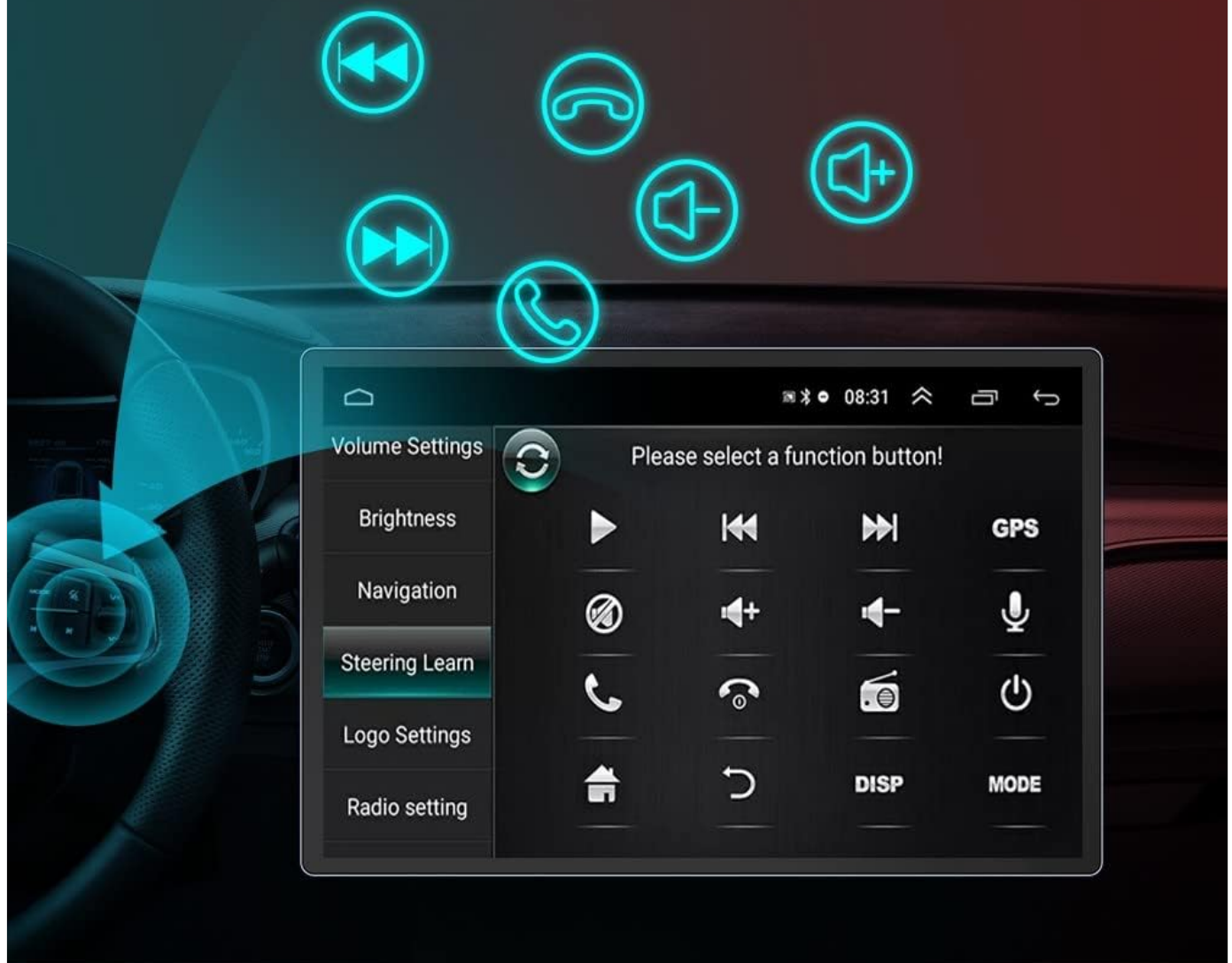
Figure 6.5: Steering Wheel Control Configuration. This image illustrates the process of mapping steering wheel buttons to headunit functions through the 'Steering Learn' menu.
