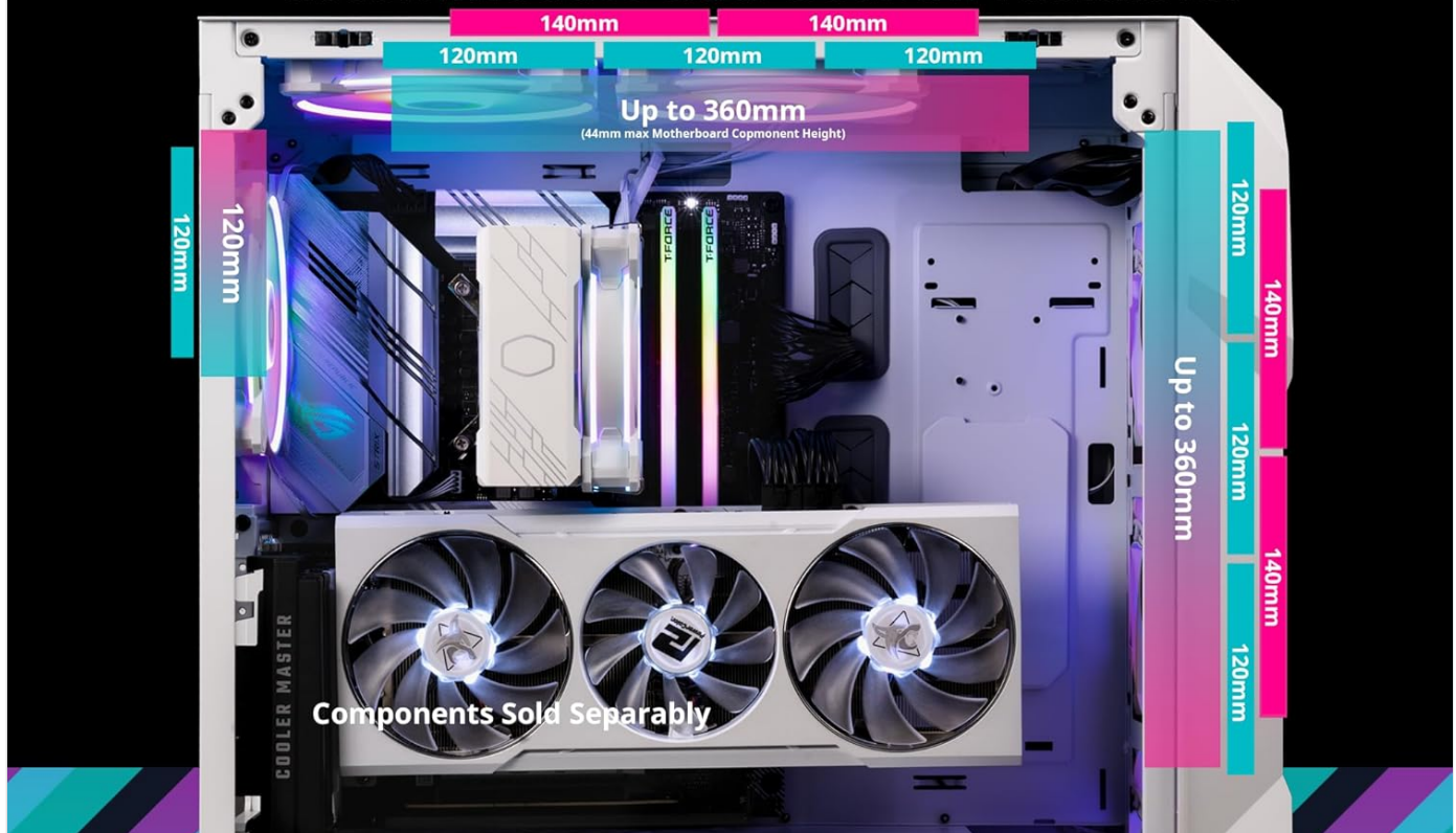
Figure 6: Overview of versatile cooling options, showing support for various fan and radiator sizes.
