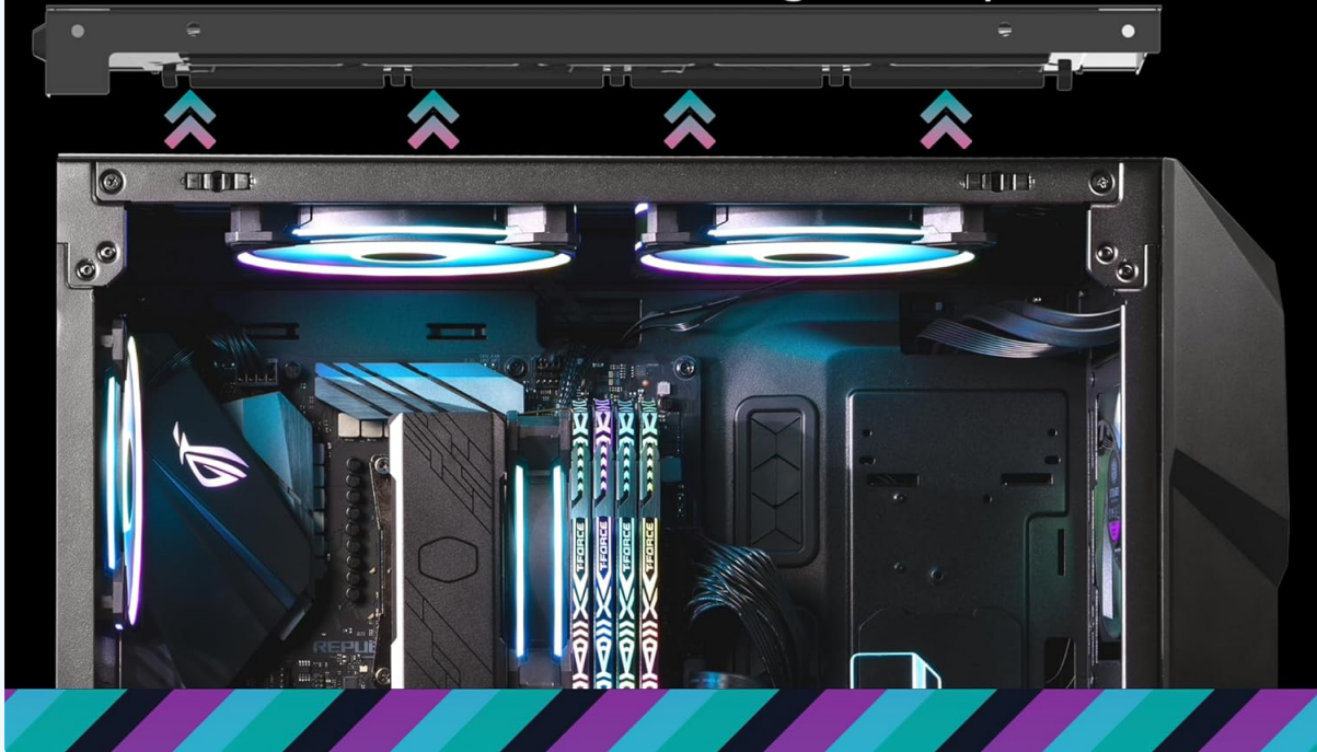
Image: The top panel detached from the case, showing the internal mounting points for fans/radiators.
