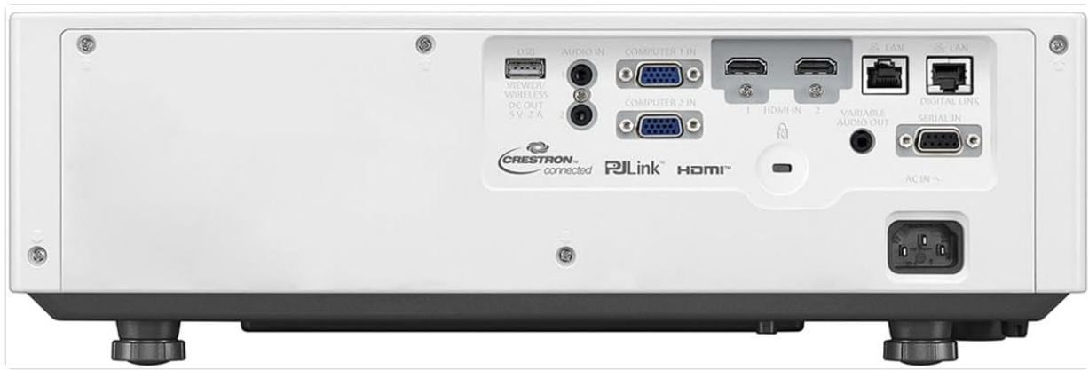
Figure 3.2: Rear panel with connectivity options including HDMI, Computer (VGA), LAN, USB, and DIGITAL LINK.
