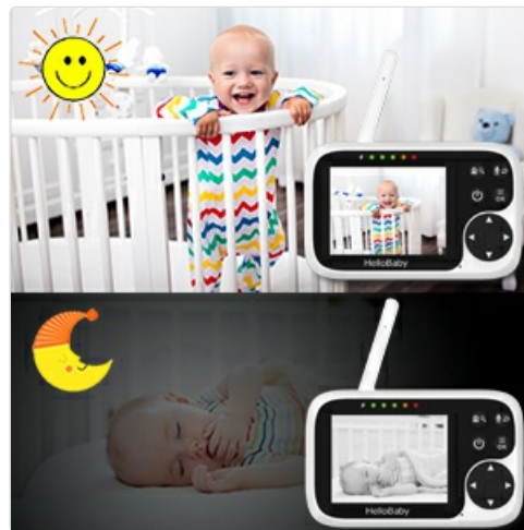
Image: Demonstration of the monitor's clear day vision and automatic IR night vision capabilities.
