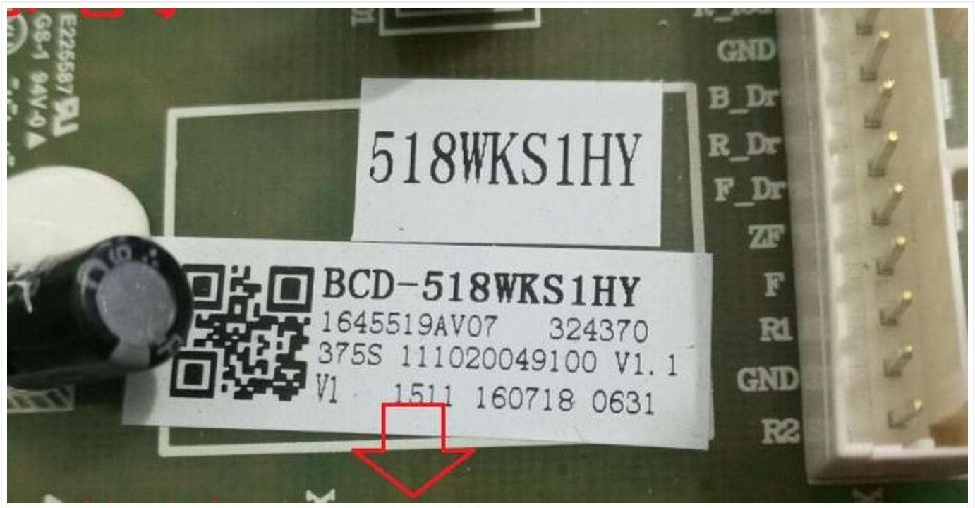
Figure 2.1: Front View of the Computer Board. This image displays the front side of the BCD-518WKS1HY refrigerator computer board. A white label is visible, clearly showing the model number "BCD-518WKS1HY" and part number "1645519AV07", along with a QR code and other manufacturing details. Various electronic components, including capacitors, resistors, and integrated circuits, are mounted on the green circuit board. Connector pins are visible on the right side for electrical connections.
