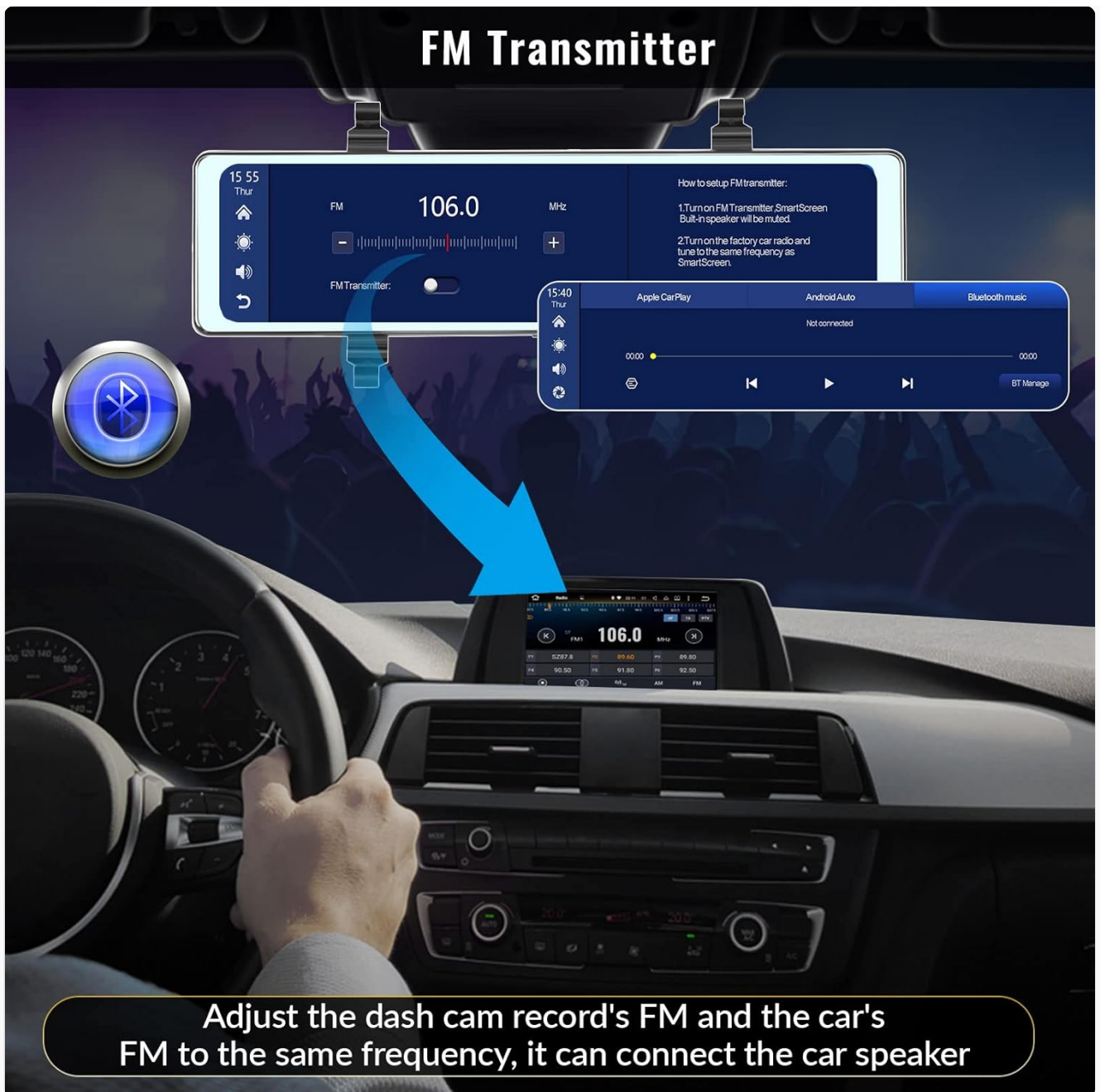
Image: An illustration demonstrating how the dash cam's FM transmitter function allows audio to be played through the car's built-in speaker system.
