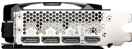
Rear I/O panel of the graphics card, featuring three DisplayPort and one HDMI output.
