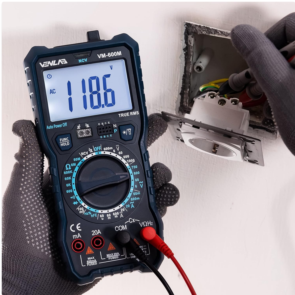
Figure 4.3: Measuring AC Voltage.
