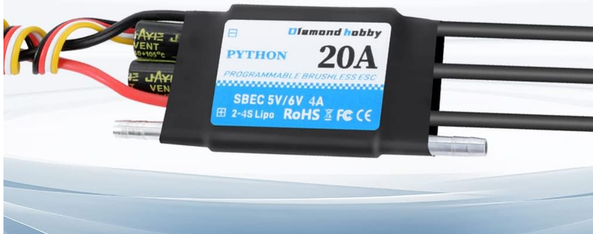
Figure 4: Illustration emphasizing the bilateral waterproof design of the ESC, suitable for marine applications.
