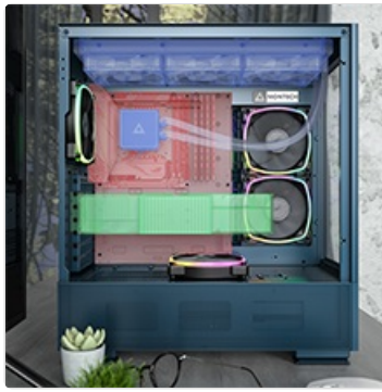
Figure 4: Diagram illustrating the optimal fan placement and airflow paths within the Montech Sky Two case for efficient cooling.
