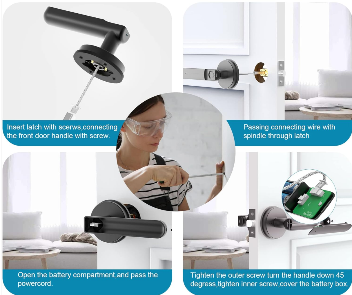
Figure 2: Visual guide for the DIY installation process, including inserting the latch, routing wires, and securing handles.
