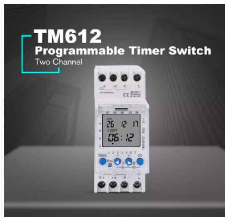
Figure 4: The TM612 timer switch, emphasizing its programmable nature and dual-channel capability.
