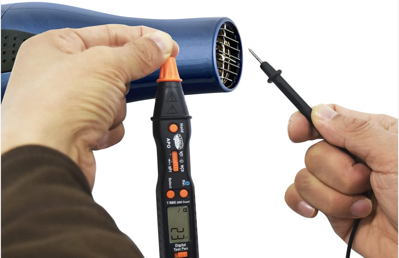
Figure 4: The multimeter displaying a voltage measurement, indicating 109V.
