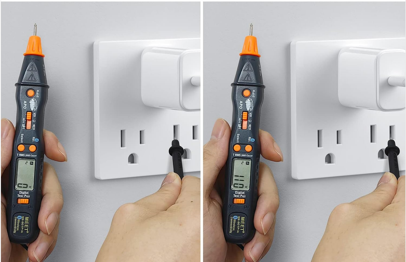
Figure 5: The multimeter's NCD function detecting AC voltage without physical contact.
