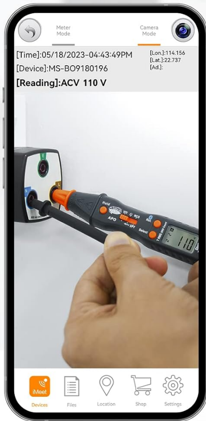
Figure 3: The multimeter transmitting data wirelessly to a smartphone application.
