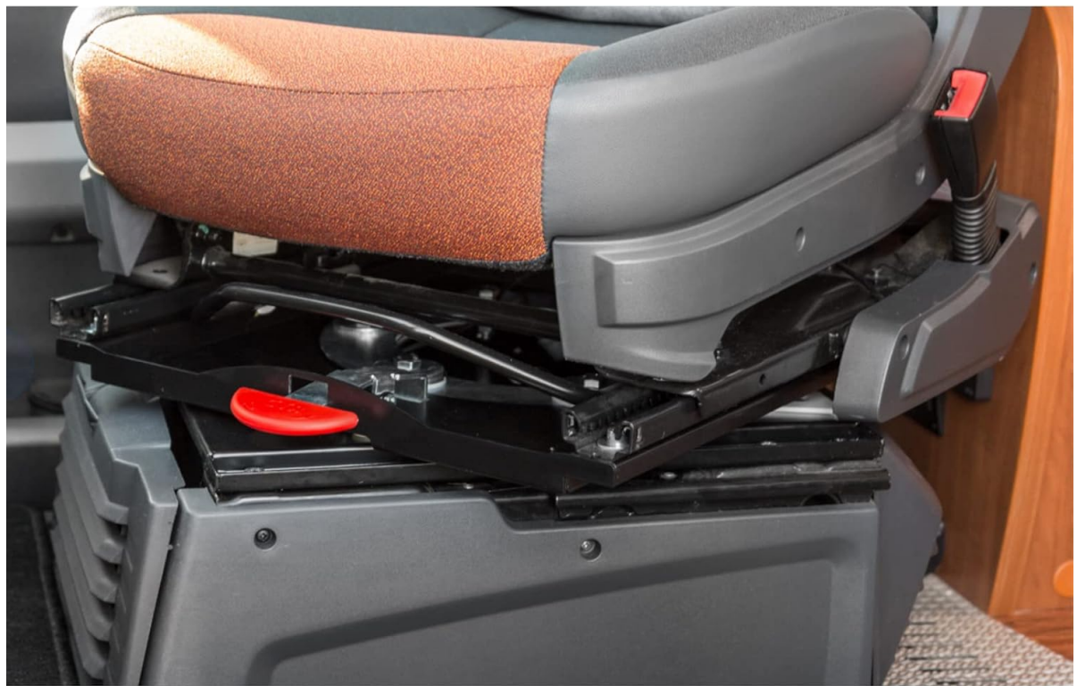
Figure 6: A vehicle seat rotated to face the rear, demonstrating the functionality of the swivel console.
