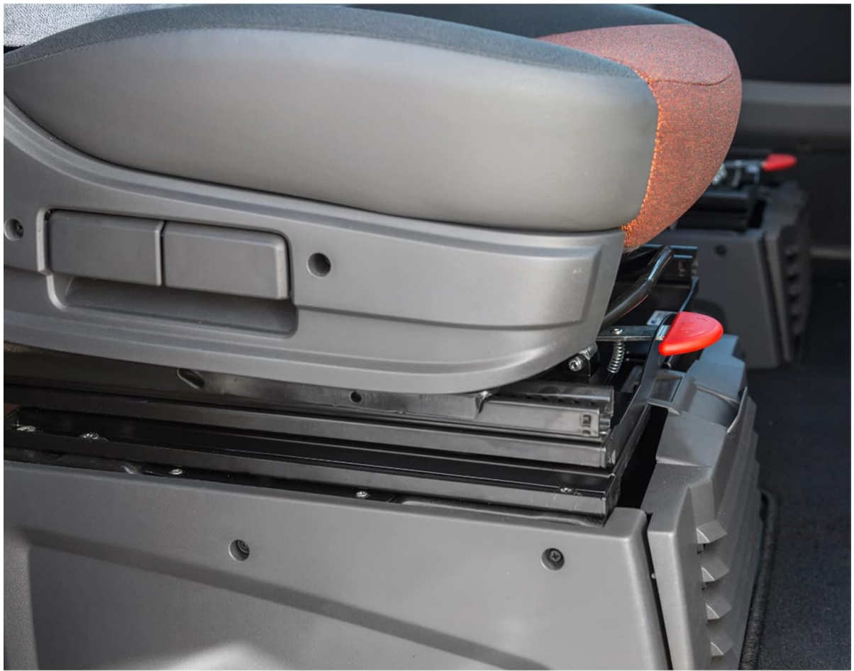
Figure 4: The swivel console integrated beneath the original vehicle seat, showing its low profile.
