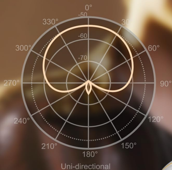
Image: Cardioid pickup pattern diagram for the TA-68 microphone.
