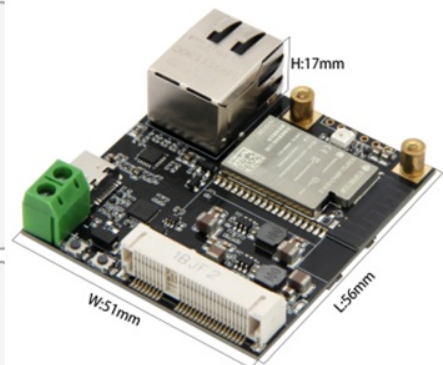
Figure 4: Module dimensions, showing approximate length, width, and height.
