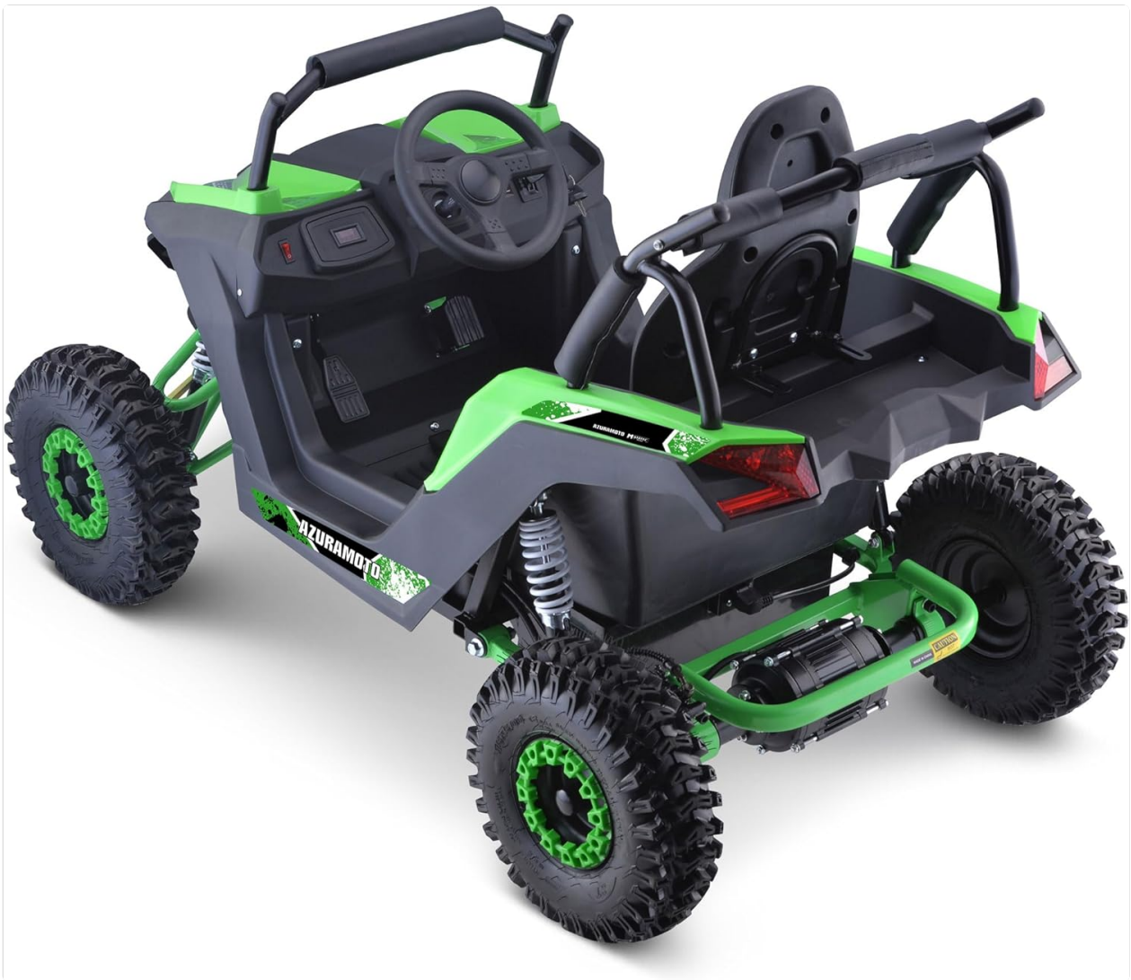
Figure 2.2: Rear 3/4 view of the MotoTec Raider Kids UTV, highlighting the rear suspension, hydraulic disc brake, and taillights.
