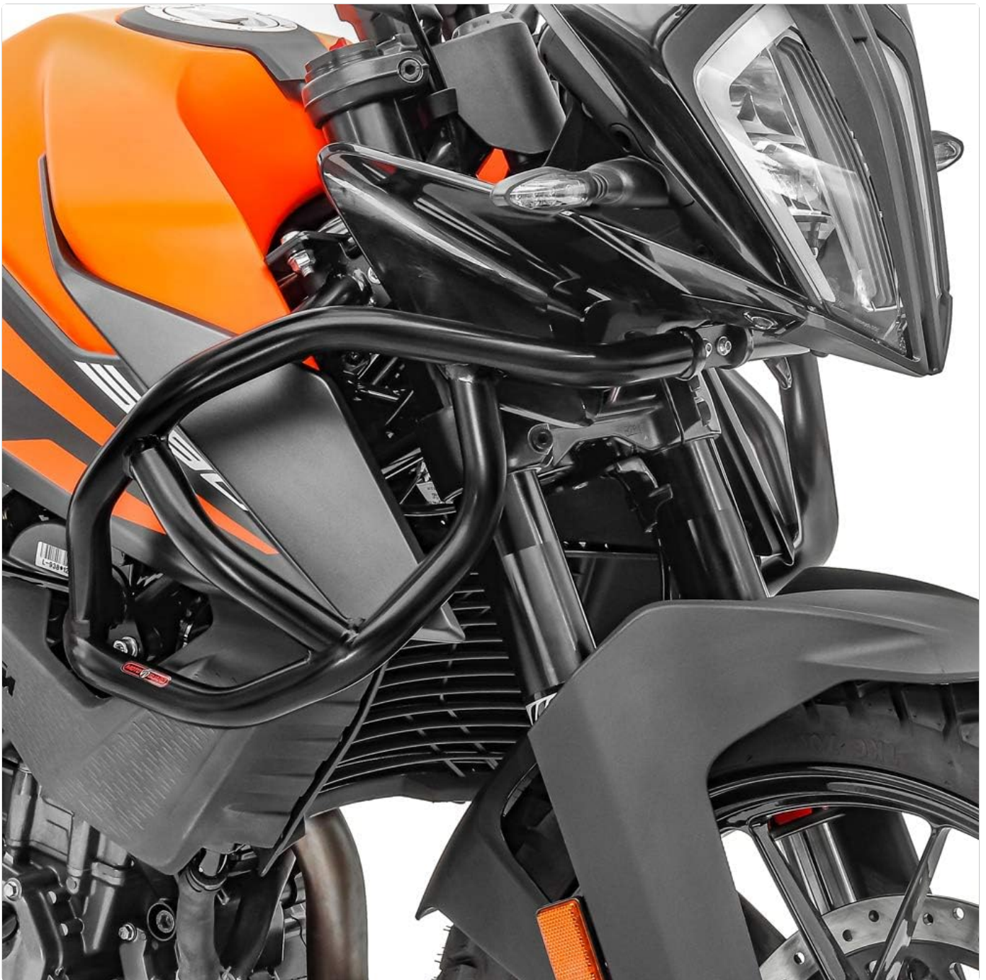
Image 5.1: Close-up view of the Motoguard DP1108 Upper Engine Guard installed on the front section of a motorcycle, showing mounting points.
