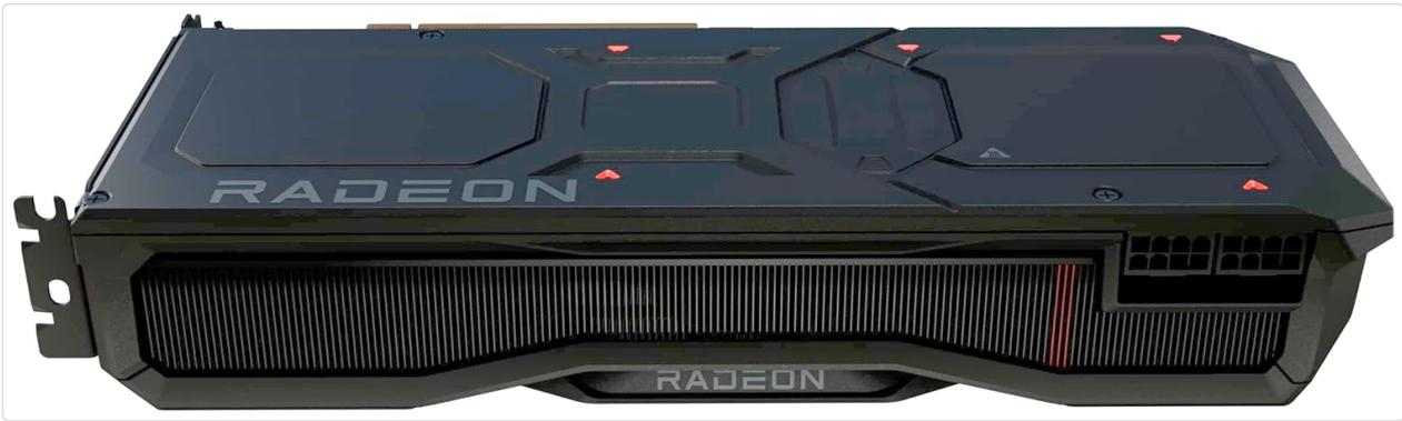
Figure 3: Top view of the graphics card, highlighting the power input connectors.
