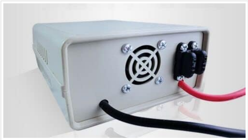
Figure 5.1: Rear view of the SUSAN 835MP, illustrating the input power cable connection point and the cooling fan.
