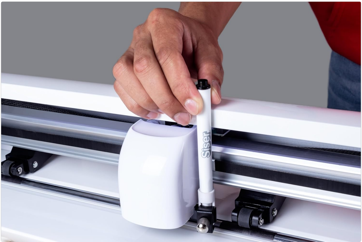
Image: Loading material into the Romeo cutter, ready for cutting or drawing with the marker adapter.
