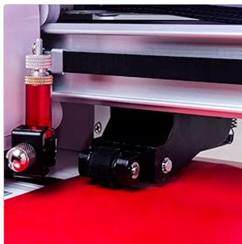
Image: Adjustable pinch rollers on the Romeo cutter, allowing for various material widths.
