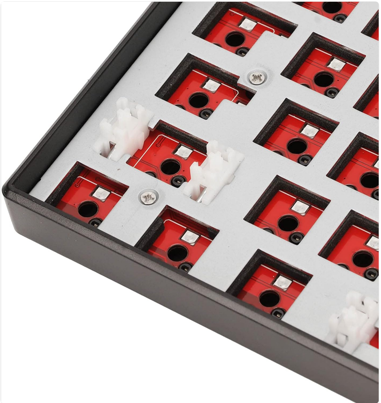
Image: A close-up view of the hot-swap sockets on the keyboard's PCB, designed for easy switch installation.
