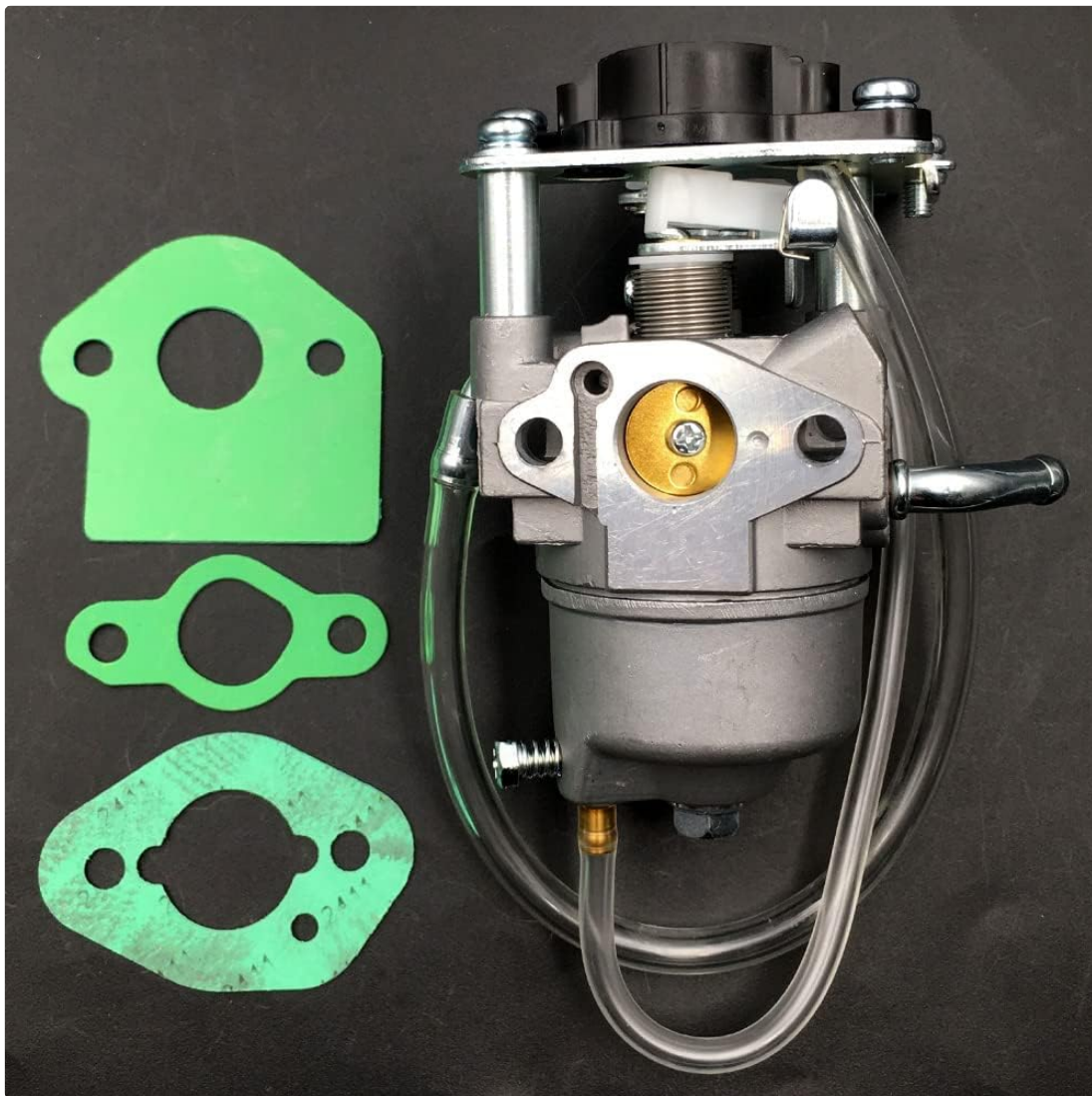
Image 3: Front view of the carburetor, showing the air intake opening and the throttle plate. The three green gaskets are visible to the left.
