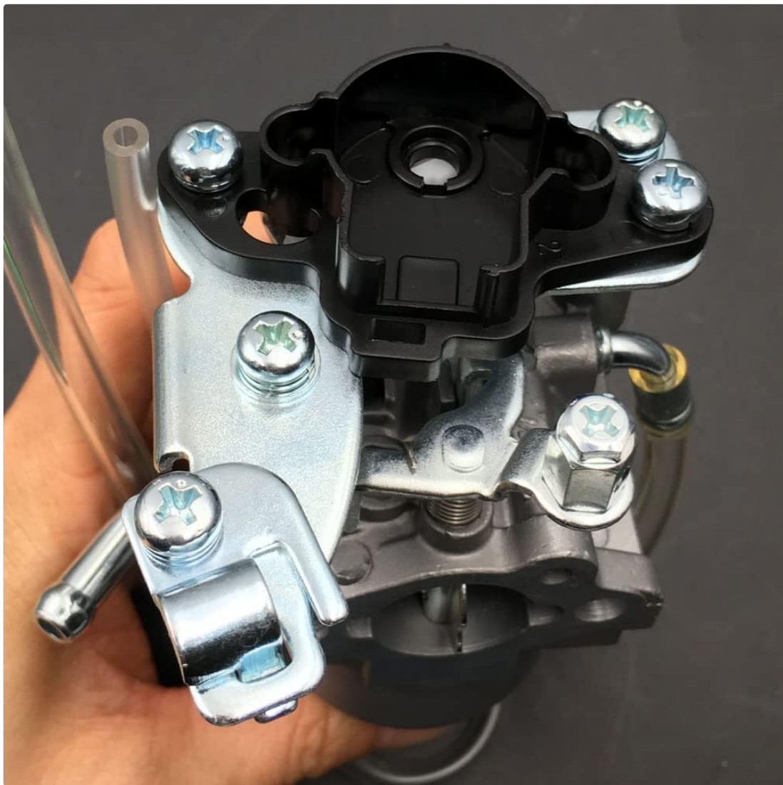
Image 6: Top view of the carburetor, illustrating the throttle linkage mechanism and mounting points. The black plastic component is part of the throttle control.
