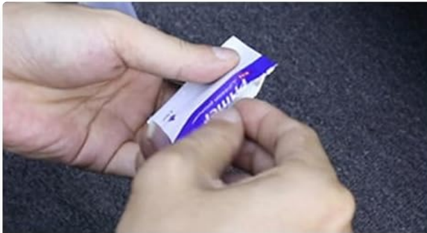
1. Wipe the doorsill with adhesion promoter.
