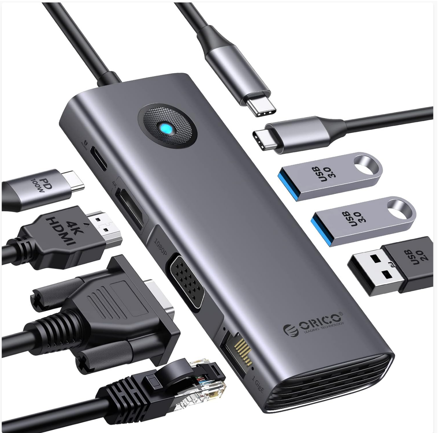
Figure 1: ORICO 8-in-1 USB C Docking Station with its various connectivity options.
