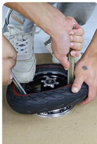
Step 3: Place either side of the hub on the tire and step on this side (Two people are recommended for installation).
