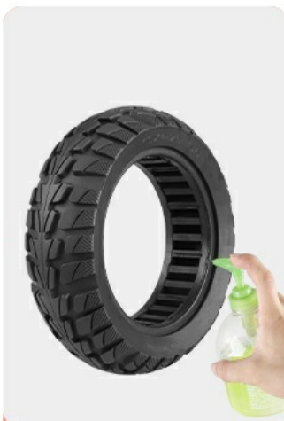
Step 2: Cover the inside of the tire with soapy water or Vaseline (Please avoid using the gasoline or lubricating oil, otherwise the tire will be damaged).
