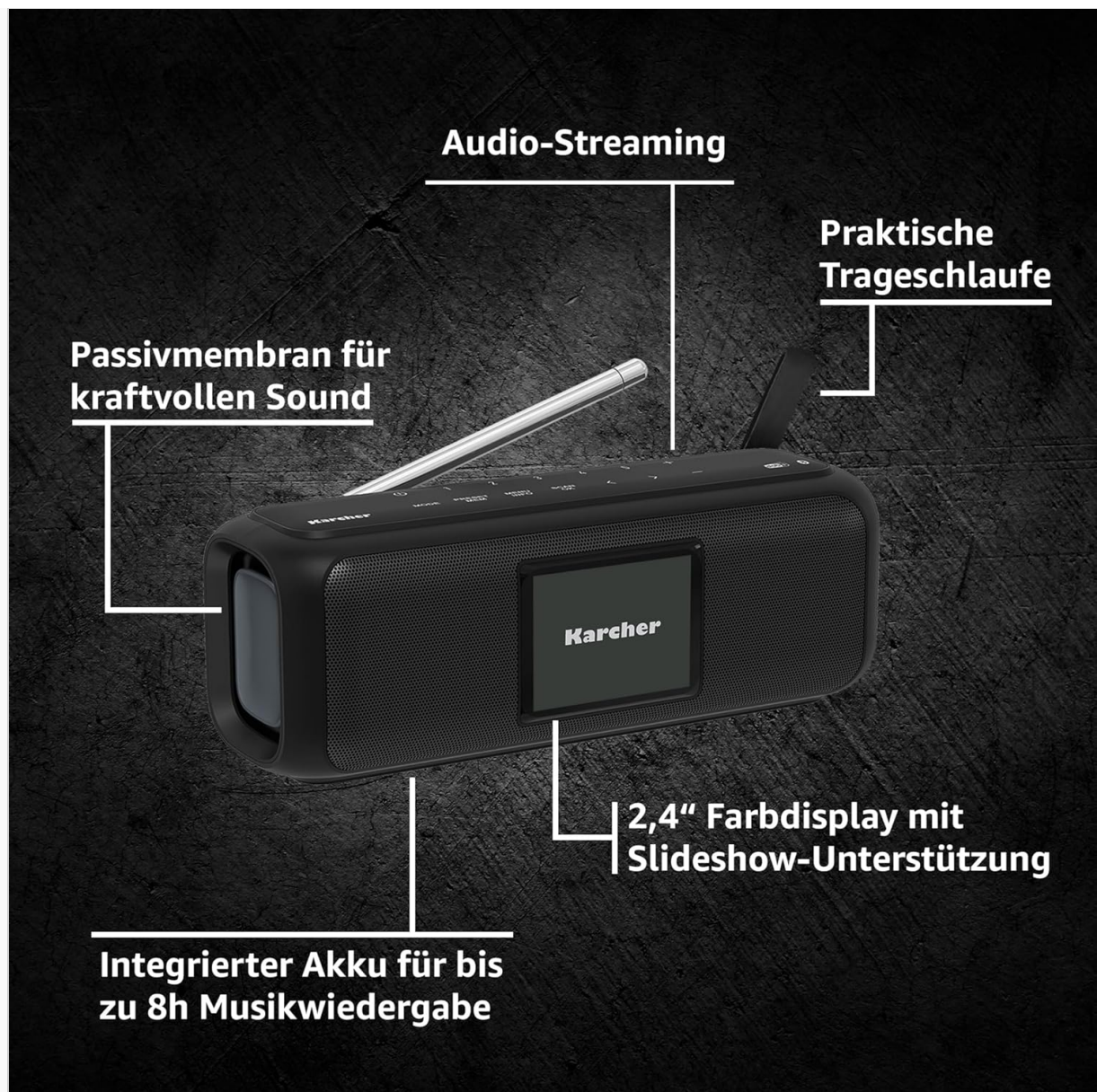
Image 3.2.1: Feature overview of the Karcher DAB Go, detailing its passive membrane for sound, practical carrying strap, 2.4-inch color display, and integrated battery for up to 8 hours of music playback.
