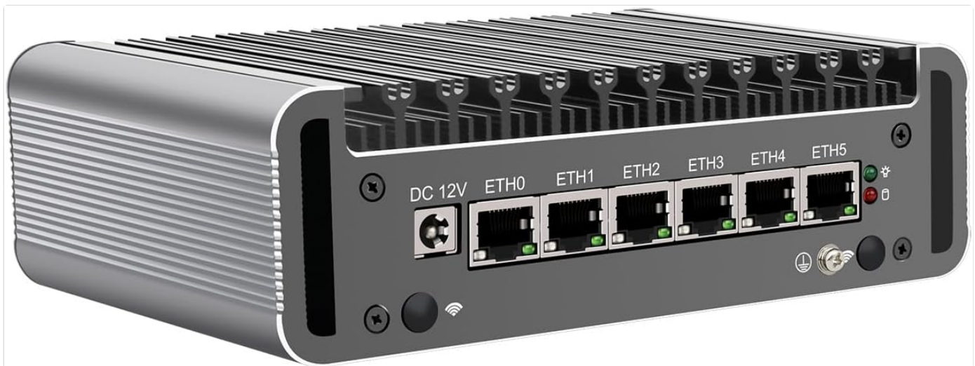
Image 3.2: Rear panel of the HUNSN RJ05f. From left to right: DC 12V power input, six 2.5GbE Ethernet ports (ETH0 to ETH5), and a SIM card slot.
