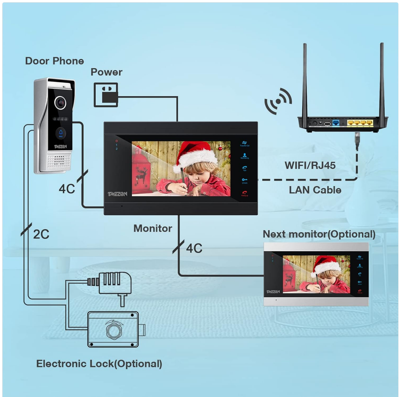
Image: Detailed wiring diagram illustrating the connections between the door phone, indoor monitor, optional electronic lock, and network router (via Wi-Fi or LAN cable). It shows 4-core cable connections for power and video stability.
