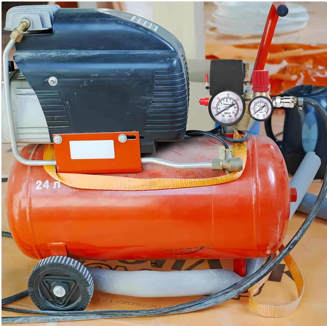
Image: Example of the pressure switch installed on an air compressor.
