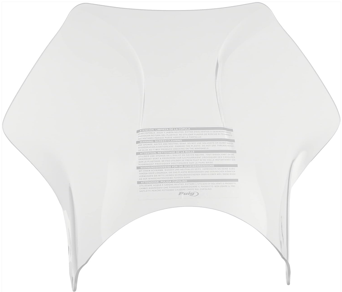
Figure 1.1: Puig Windshield Raptor (Clear). This image displays the clear polycarbonate windshield, which is designed to deflect wind and enhance the motorcycle's aesthetics. A warning label regarding cleaning is visible on the surface.
