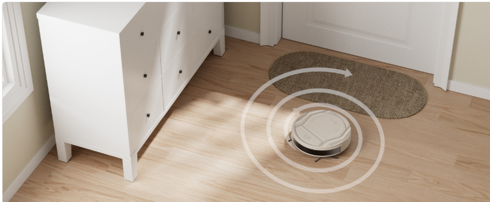
Image: The robot vacuum performing spot cleaning, moving in a spiral motion to thoroughly clean a concentrated dirty area on the floor.
