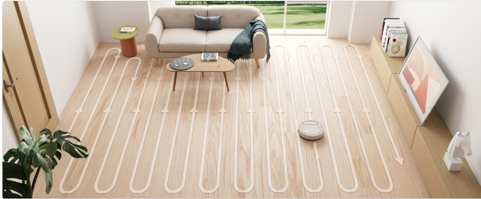
Image: An illustration showing the robot vacuum cleaning a room in a systematic zigzag pattern, which is effective for covering large open areas and minimizing missed spots.
