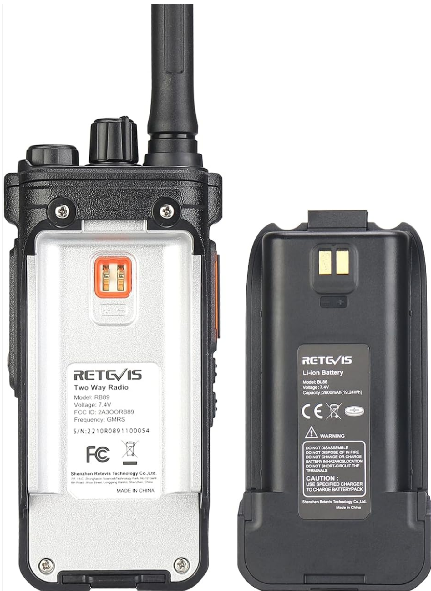
Rear view of the RB89 radio with battery details and regulatory information.
