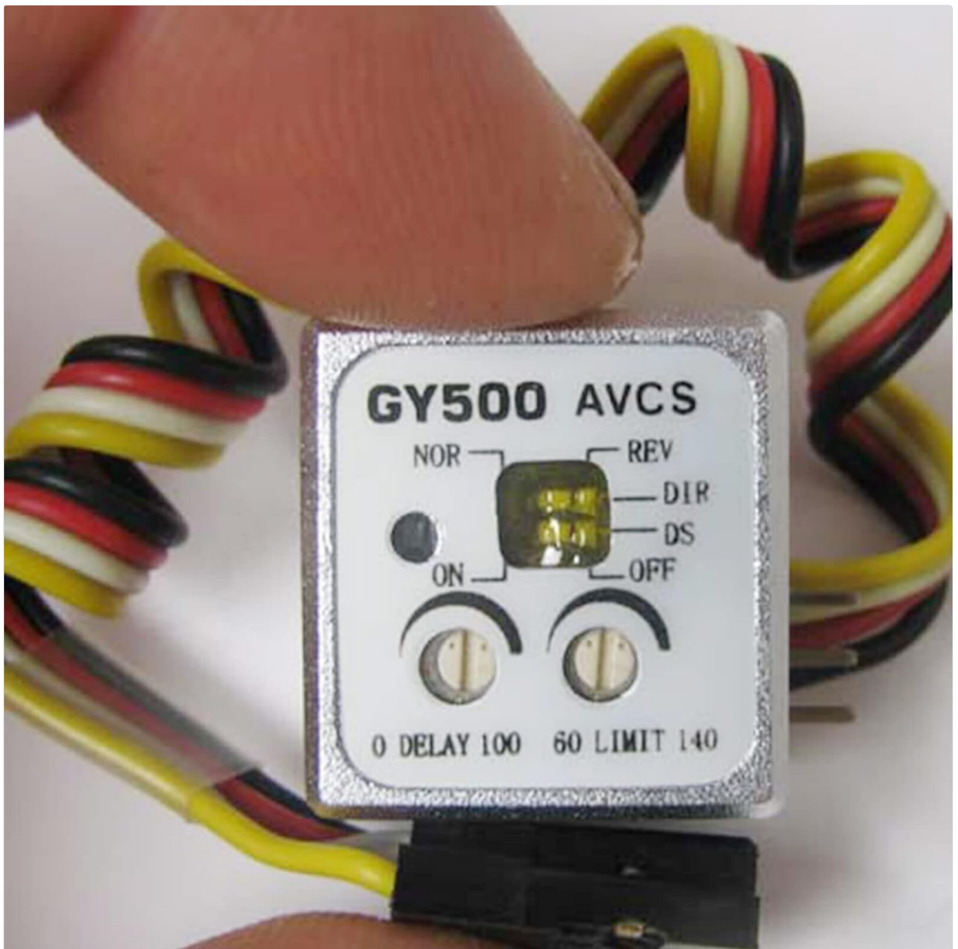
Image: A close-up view of the GY500 gyro, highlighting its control panel and the attached wiring harnesses.
