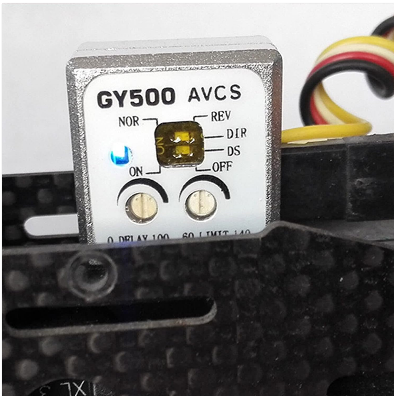
Image: The GY500 gyro mounted on an RC helicopter frame, showing its compact size and placement.
