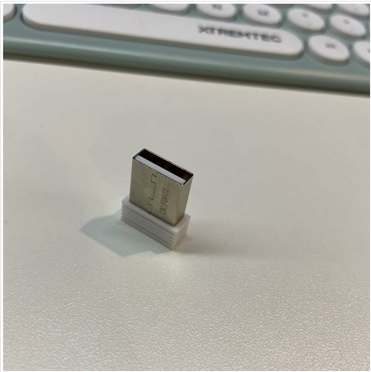
Image: The Mobifice K101B USB Adapter, a compact device with a USB Type-A connector, shown ready for connection to a computer. This adapter facilitates USB connectivity for compatible keyboards.
